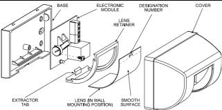
Figure 9. DA-5 Exploded View
