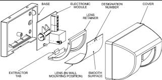
Figure 9. DA-5 Exploded View
