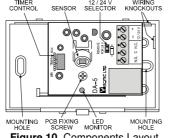
Figure 10. Components Layout
